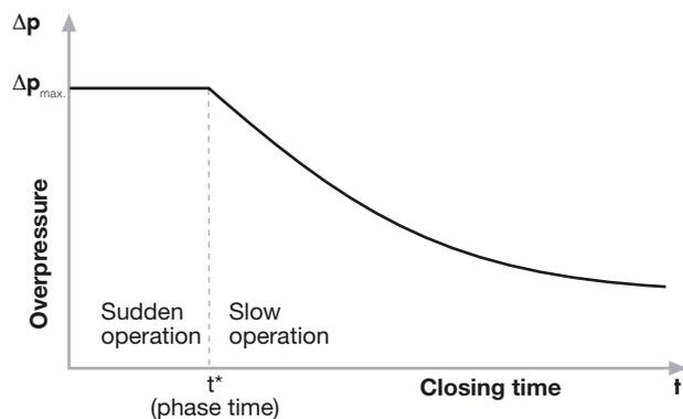
Numerical example: pipe length 10 m, diameter equivalent to 1/2", steel, copper and PE-X pipes with water velocity  $v_1 = 2$  m/s. We give the values of the velocity of the perturbation propagation  $v_2$ , sudden operating times  $t^*$  (phase time) and the overpressure  $\Delta p$  obtained with the formulas.
