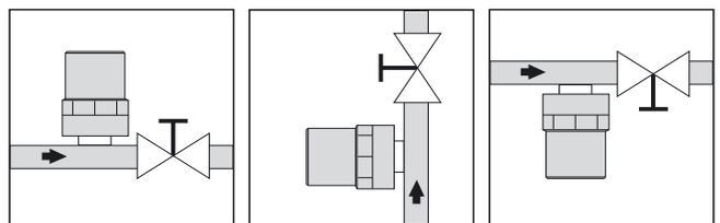
The Caleffi 525 series water hammer arrester must be installed as close as possible to the device which gives rise to the water hammer by suddenly shutting off the water flow, so as to damp the resulting overpressure as soon as possible. It may be installed horizontally, vertically or upside down.
