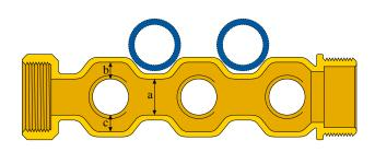
The partial pipe housing in the manifold outline is also helped by the fastening brackets, which are made with an angle that provides a 25 mm offset between the upper and lower manifolds.
