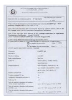
The bench calibration report is the document confirming the testing of each individual device included in the approved series. The test is carried out in the presence of an I.S.P.E.S.L. inspector who draws up the report after the test has been passed. The document gives the serial number of the valve, which is also to be found on the plate fixed to the valve body.
