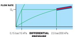
$Kv_{0.01} = 0,070 \cdot G_0$  range  $\Delta p$  15–200 kPa where  $G_0 = nominal$  flow rate
