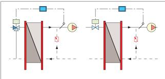
To create heat exchanger flow balancing by-passes
