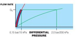
$Kv_{0.01} = 0,258 \cdot G_0$  range  $\Delta p \ 15-200 \text{ kPa}$  where  $G_0 = nominal$  flow rate
