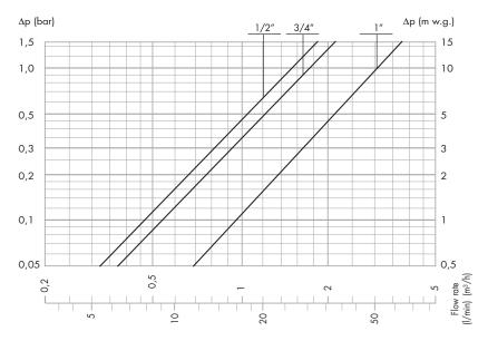
Recommended flow rate values to ensure stable operation with an accuracy of  $\pm 2^{\circ}C$
