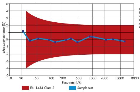
SENSONICAL ULTRA is a MID certified heat meter with accuracy level 2 in accordance with EN 1434. The graph alongside plots the error curve of a specimen meter (blue curve) and the limits imposed by class 2 (red area).
