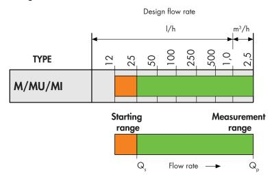
The decisive factors to select a heat meter are the design flow rate, i.e. the theoretical minimum and maximum quantity of water circulated. The maximum possible flow rate must be equal to or less than the nominal flow rate  $(q_p)$ . The minimum flow rate must be greater than the lower limit of the measurement range  $(q_i)$ .
