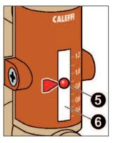
4) After completing the balancing, release the ring of the flow meter obturator (2) that, thanks to an internal spring, will automatically go back into the closed position.
