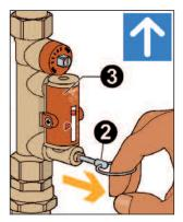
3) Keeping the obturator open, use a 9 mm hexagonal wrench on the valve control stem (4) to adjust the flow rate. It is indicated by a metal ball (5) that runs inside a transparent guide (6) marked by a graduated scale in m<sup>3</sup>/h alongside it.
