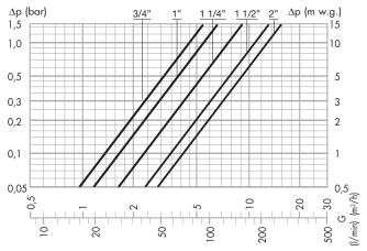
Recommended FLOW RATES to ensure stable operation and accuracy of ± 2°C (balanced Hot/Cold pressures)
