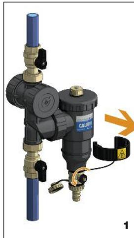
Remove the ring in which the magnets are housed (fig.1) and drain the impurities, even while the system is running, using the special key provided (fig.2).
