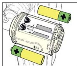
Electric supply is provided by two 1,5 V AA batteries with lifetime of up to 2 years depending on use.
