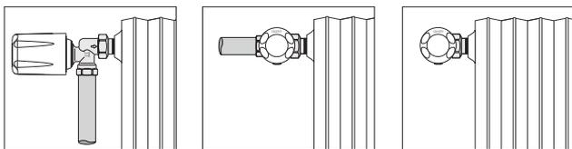
The electronic control heads **must be installed in a horizontal position** to allow a correct temperature reading to the internal sensor. If this proves impossible (e.g. a control head installed in a horizontal position would obstruct opening of a door) it becomes mandatory to use the ambient temperature sensor to replace the internal sensor in the control head. In this case the control head can be installed in a vertical position if necessary.
