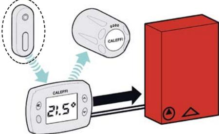
The temperature sensor is optional in that the electronic control head is already equipped with a built-in temperature sensor. Use of the sensor is recommended in the case of installation in conditions that could impair correct temperature readings. E.g., under deep shelves, as shown in the figure.
