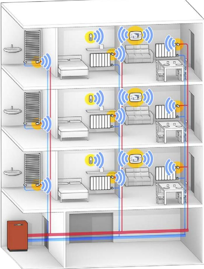
The controller receives the signal from the temperature sensor to establish the presence of heating demand in the zone in question on the basis of the programming. The valves located in the zone in question are adjusted accordingly.
