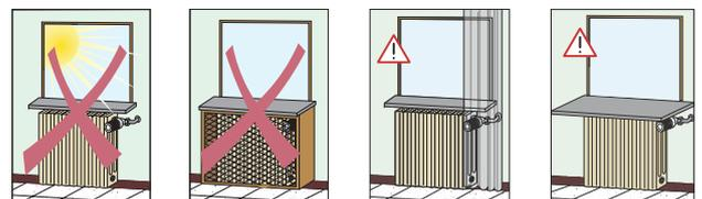
**It is good practice** to install an ambient temperature sensor in each zone if radiators are installed in recesses, in cabinets, behind curtains, under deep shelves, or exposed to direct sunlight thus creating conditions that could affect the accuracy of temperature readings.
