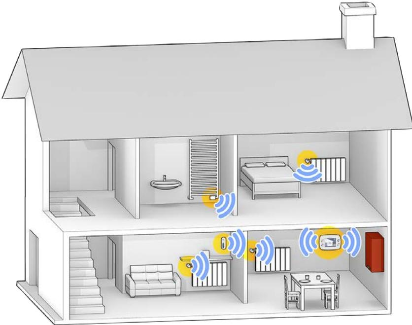
The controller receives the signal from the temperature sensor to establish the presence of heating demand in the zone in question on the basis of the programming. The valves located in the zone in question are adjusted accordingly. The boiler is started by means of the specific relay output in the presence of a heating demand from at least one of the zones.
