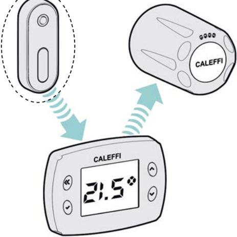
The temperature sensor is optional in that the electronic control head is already equipped with a built-in temperature sensor. Use of the sensor is recommended in the case of installation in conditions that could impair correct temperature readings. E.g., under deep shelves, as shown in the figure.
