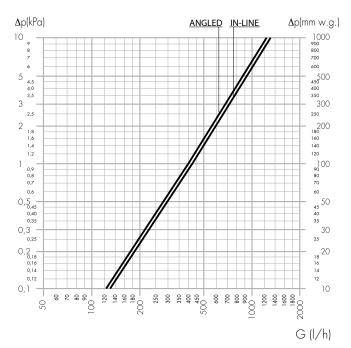
Kv (m<sup>3</sup>/h) with in-line configuration = 4,2 Kv (m<sup>3</sup>/h) with angled configuration = 3,9 Maximum recommended flow rate = 1,3 m<sup>3</sup>/h
