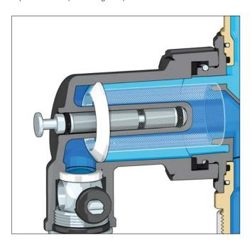
It is possible to drain the impurities without disassembling the body, just by removing the magnet and opening the dedicated cock. Only perform this operation when the system is not in operation.
